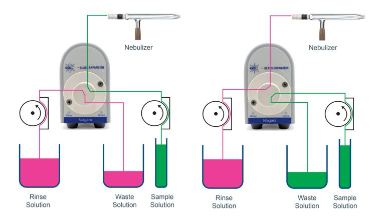
During the read time (Figure 1) the rinse solution is pumped through the valve to waste.
